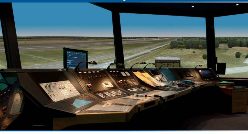
e.sigma Solutions for Air Traffic Control Training (CBAST™) are proven and modular systems for civil and military ATC training requirements. The system architecture allows the scaling of controller, instructor and pseudo pilot positions, as well as tower visual systems from office-room size to large scale training centers.
